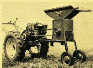
Model 5-N with stabilizer bar attached to garden tractor. Model 5-G with 2 1/2-hp gas engine. Model 5-E with 3/4-hp electric motor.
