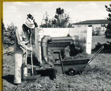
Model 4-M Shredder-Grinder only with standard 35" x 36" hopper and 9-hp engine.
